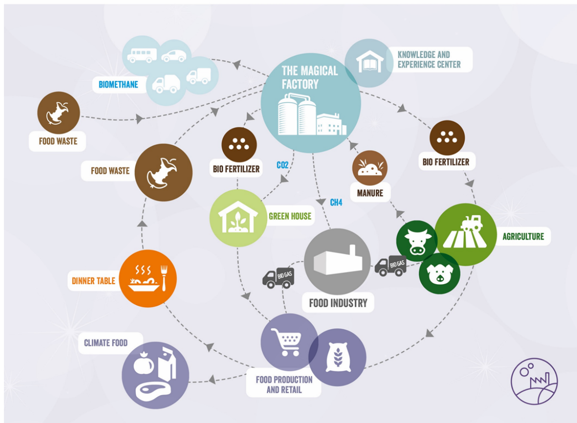
Figure 3. An example of a circular concept which creates synergies and benefits for all parties involved. The Magic Factory (2023) is a biogas plant in Norway receiving municipal and commercial source separated food waste as well as manures from cow, pig and fish. The output is biomethane (CBG, which fuels public buses, trucks and local food industry, and LBG, serving more distant markets), biofertiliser (digestate), which has substituted most of the mineral fertiliser in the area, and CO 2 , which is used in a greenhouse.
